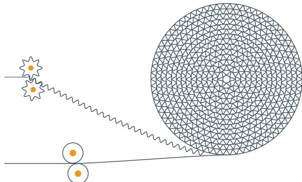
As well height (gap between wraps) increases, the amount of heat transfer and pressure drop is reduced. The decrease in well height increases the transfer of heat and pressure drop. In EVO Modular Air Handling Units, condensing type rotors with a 1.6 mm well height are used as standard. For higher heat transfer requirements, rotors with 1.8 mm, 2.0 mm or 2.5 mm well height can be selected from the selection software for 1.4 mm can be chosen for lower pressure drop requirements.
