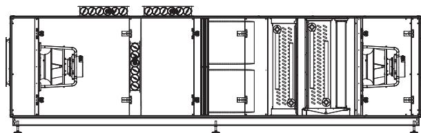
For air flow adjustment, a resistance is created in the economizer damper and the return air / fresh air ratio in the mixing air is adjusted according to the pressure drop created. The AERA Selection software automatically calculates the mixture air conditions according to the outside air conditions and mixing ratios specified by the user when the economizer section is selected. This information is automatically transferred to next section such as filter, battery, fan etc.
