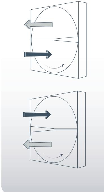
By selecting the configuration as shown in the figure in EVO Modular Air Handling Units, the static pressure values between the two air flows on the rotor will be very close to each other, so the leakage between the flows will be minimized. It is advisable to configure the units this way in modular air handling units just like compact units.
