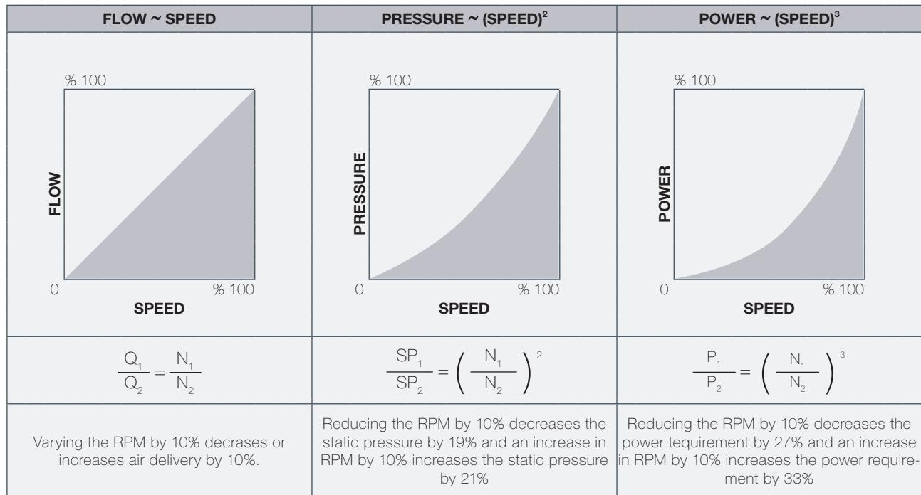
Q - Flow, SP - Pressure, P - Power (kW) ve N - Speed (RPM)
