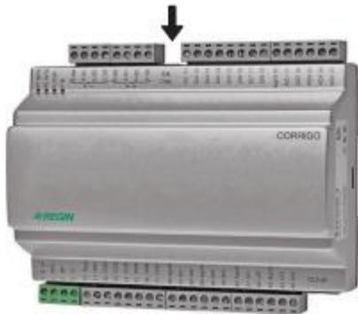
When using this mounting, the cable should be led through the alternate outlet at the bottom of the wiring compartment
