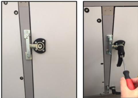
The door handles are packaged separately to avoid damage during the transport. Install the door handles after the unit is placed on floor and leveled.
