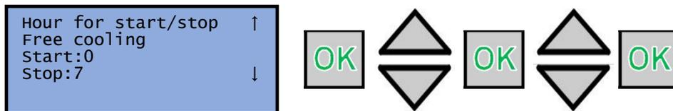
Free cooling is used to set the start and end time. Start and end times, OK key is pressed, “UP-DOWN” buttons are set, and then press “OK” button. Free cooling is started if all operating conditions have occurred within the set times.
