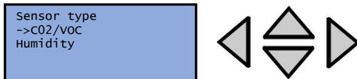
In the sensor type menu is entered by “RIGHT” direction button. With the “OK” button Reduced and boost and difference and stop time can set by the “UP-DOWN” direction buttons and press “OK” to confirm.
