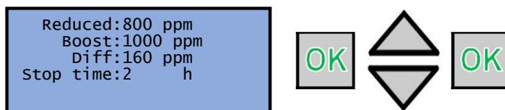
Press “OK “ button to enter the selected air quality sensor, reduced ventilation requirement, boost ventilation requirement, difference and stop time set values. Then press the “UP-DOWN” keys to set the desired values and press “OK” to confirm.
